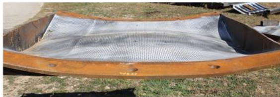
Figure 5: Post-test image of the deformed panel. The visible upper surface contains the black dot pattern for the DIC measurements on the white-painted inner hull surface.
