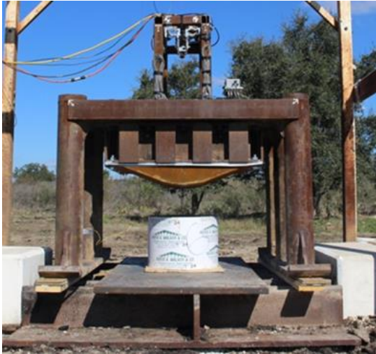
Figure 1: SwRI's Landmine Test Fixture holding a hull component above a soil pot. At the top of the test fixture is the superstructure holding dual offset high-resolution high-speed cameras.
